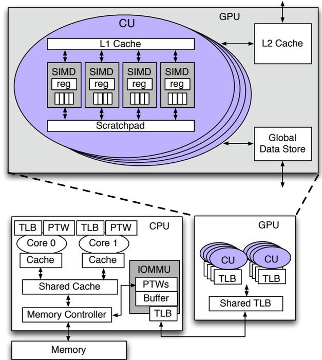
Fig. 1: Baseline Heterogeneous System Architecture.
